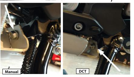
**Manual:** Use OEM Honda M8 x 18mm long bolt from step 2, plus the M8 flange nut. Attach the skid plate to the frame mount as shown, thread nut on then leave loose for now. 12mm and 13mm combination wrenches required.
