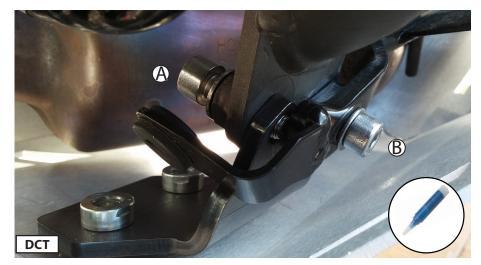
**DCT:** Install left front bracket as shown. AltRider Bracket sits against frame, with DCT guard bar stacked on top. Apply loctite to these bolts. From backside, insert M8 x 20 bolt (A) and tighten to 10Nm. This acts as as support pin to the AltRider bracket. Use M8 x 25 bolt from outside (B), through both DCT bar and altrider bracket. Do not fully tighten this bolt yet.
