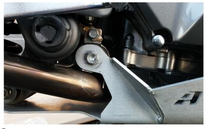
(1) Attach the left rear mount of the skid using the exhaust hanger bolt. (12mm socket). Leave loose for now.
