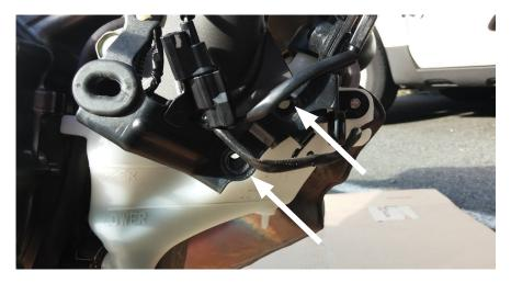
② Use 12mm wrench, remove two M8 bolts from from right side brackets on frame mount as shown. Leave brackets in place. Save the bolts for use later.
