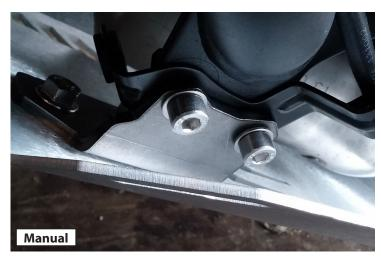
Manual Transmission: Install left front bracket as shown. Note orientation of bracket. Attach with M8 screws (one M8 x 25, one M8 x 20), tighten to 19 Nm.
