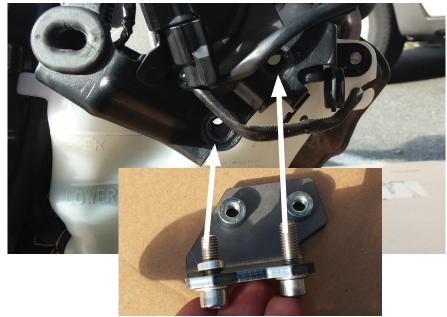
(6) Install right front bracket as shown. Stack spacer in between AltRider bracket and Honda bracket. Attach with M8x 25 screws, torque to 19 Nm. Do not pinch wires.
