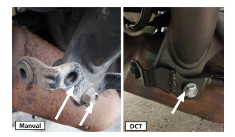
3 **Manual Transmission:** Remove two M8 bolts from left side front bracket on frame mount as shown.
